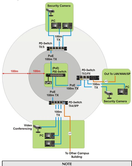
This product must be connected to PoE networks and is not intended for connection to outside plant installations.
